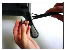
Locate the rubber grip at the end of the leg and, with your thumb, peel it back and pull it off.
