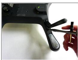
Locate the leg and remove the two 10mm screws that hold the leg in place.
