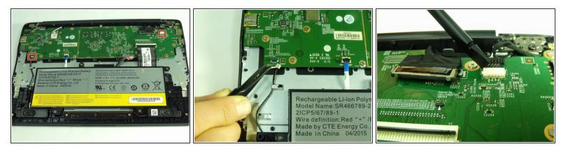
• Disconnect the speaker and charging port cables by pulling the connectors out of their sockets.
