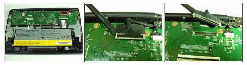
• Disconnect the LCD screen connector from the motherboard using a spudger.
