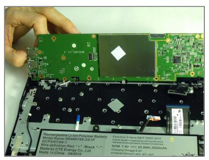
• Lift and remove the motherboard away from the frame.
