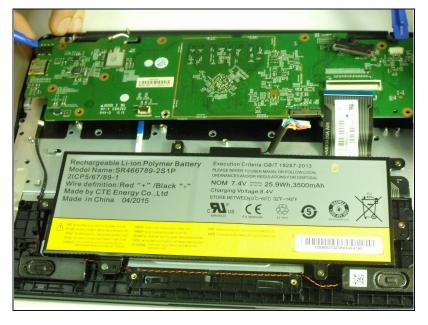
Use a plastic opening tool and pry around the edges of the motherboard to release.
