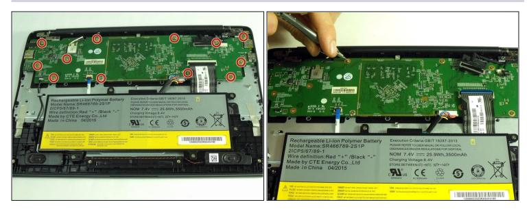
• Use a #000 Phillips screwdriver and remove the twelve 4mm screws that hold the motherboard.
