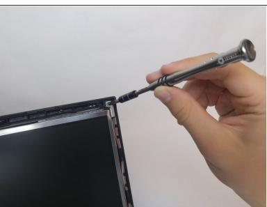
Use a Philips #0 head screwdriver to remove the two 6.0mm screws from the top corners of the LCD screen.
