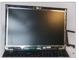
• Continue along the edges lifting up and prying off the plastic LCD bezel.
