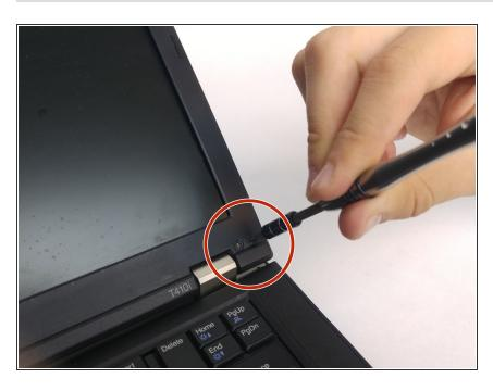
Remove the two 6.0mm screws on each side using Philips #0 head screwdriver as shown in the picture.
