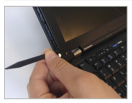
Use a spudger to separate the bezel of the LCD screen.
