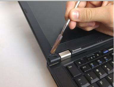
Use a spudger to remove the plastic covers from the LCD screen.
