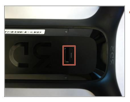
Locate the release button on top of the battery.
