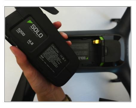
Lift the battery from the drone.
