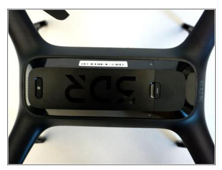
Lay the drone down on its legs so that the power button is facing up.
