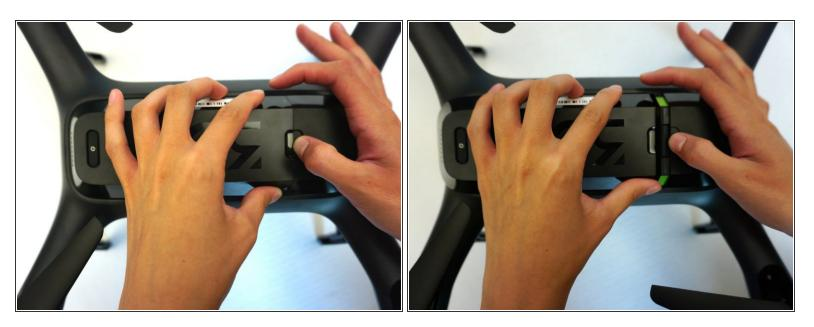
With one finger, push down on the release button and with the other, grip the battery and slide it to the left.
