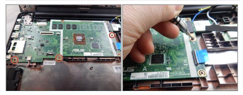
• Remove the three 3.0mm Phillips #00 screws that secure the motherboard to the housing.
