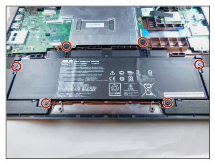
• Remove the six 6.0mm Phillips #00 screws that secure the battery to the bottom housing.
