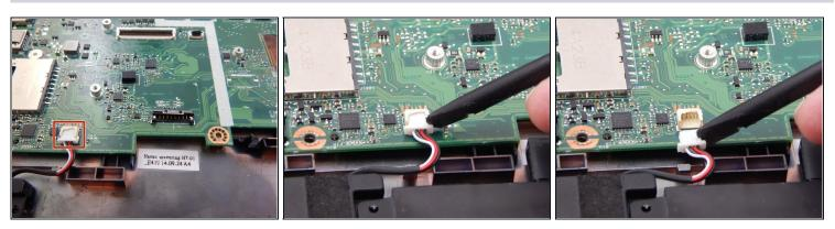
• Disconnect the speaker cable from the motherboard using the plastic spudger tool.
