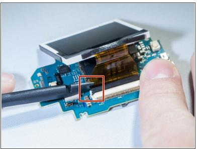
Undo the ribbon cable attached between the motherboard and screen by prying up black tab which holds the cable, using spudger. (See pictures)
