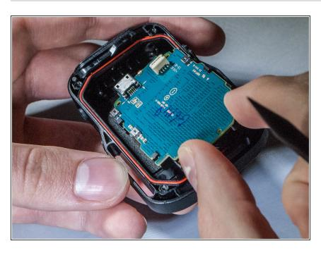
Remove motherboard from the device by pulling upward gently, with fingers or tweezers.
