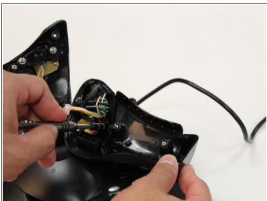
Remove the two 8 mm J1 JIS head screws.
