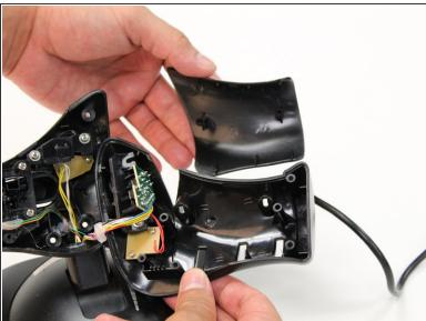
Remove exterior panel from the throttle by using your hands to gently pull the panel away.
