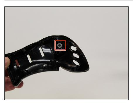
Once the black panel is disconnected, push the triangle button inward from the outside of the exterior panel.
