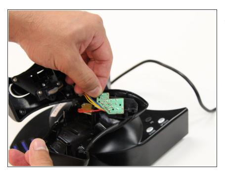
Carefully remove the circuit board.
