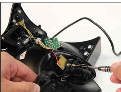
Remove the 6 mm J1 JIS head screw that is attached to the black plastic cover.
