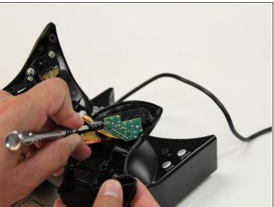
Remove the two 6 mm J1 JIS head screws from the circuit board.
