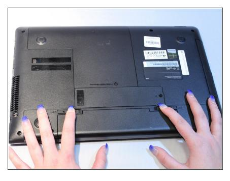
Slide the left and right switches to the unlock position.
