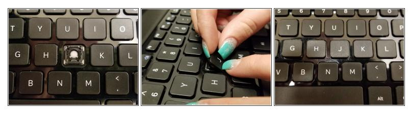
Once the retainer is attached, press the key onto the retainer, it will make a snapping sound when in place.
