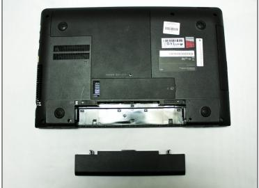
While holding the left and right lock switches in the unlock position, pull the battery away from the computer.
