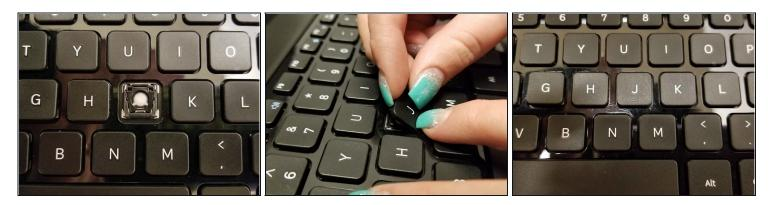
• Once the retainer is attached, press the key onto the retainer, it will make a snapping sound when in place.
