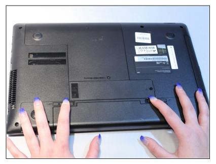
• Slide the left and right switches to the unlock position.
