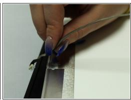
Locate and remove the tape from the back of the display in the two (2) sections marked on the supporting image.
