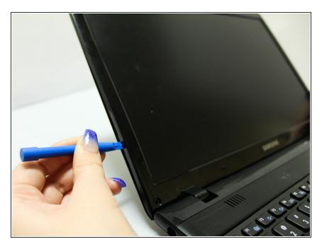
Carefully pry the front display cover off with a plastic prying tool.
