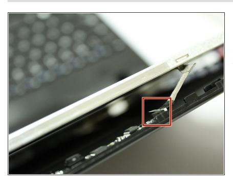
Carefully remove the connector between the display and the display casing by pulling the connector away from its outlet.
