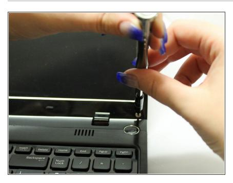
Remove the two (2) 2.27 mm screws with the Philips #0 screwdriver.
