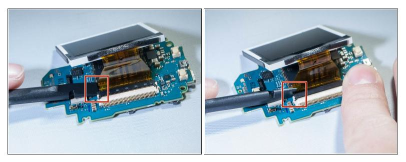
• Undo the ribbon cable attached between the motherboard and screen by prying up black tab which holds the cable, using spudger. (See pictures)
