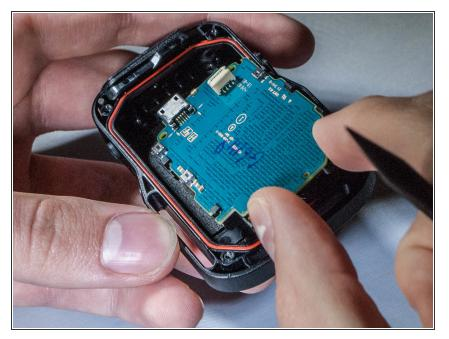
Remove motherboard from the device by pulling upward gently, with fingers or tweezers.
