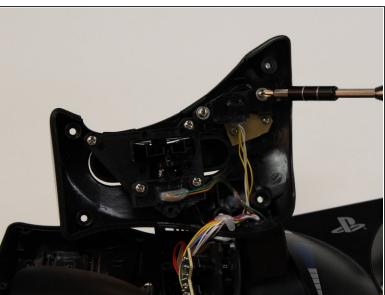
Remove the two 7 mm J1 JIS head screws from the panel covering the buttons.
