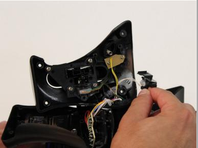
Pull the panel that is covering the R2 button away from the throttle.
