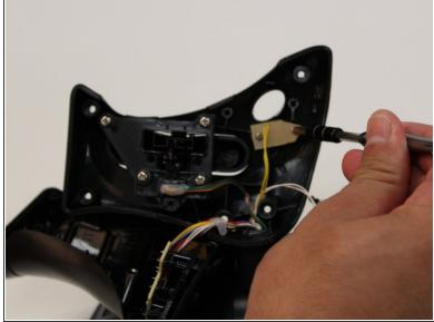
Remove the two 4 mm J1 JIS head screws from the panel covering the L2 button.
