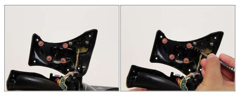
• Remove the four 13 mm J1 JIS head screws from the rudder assembly holder.
