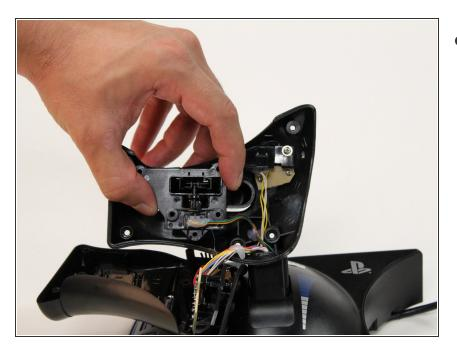
• Gently remove the panel that is covering the rudder.
