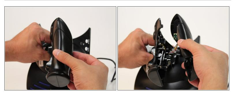
(i) Be sure to disconnect the controller from the power source before disassembling.
