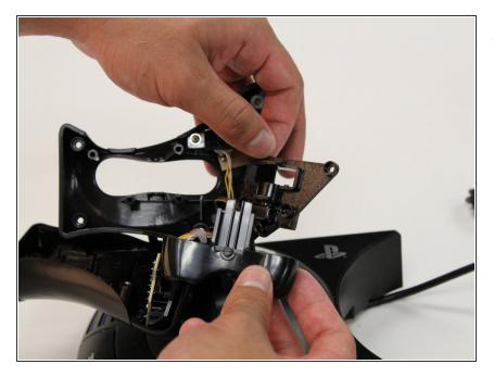
• Proceed to remove the rudder from the throttle.
