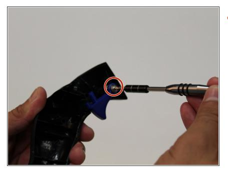
Remove the 8 mm J1 JIS head screw that is holding the trigger in place.
