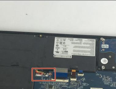
After opening the bottom plate, locate the battery and the battery connection.
