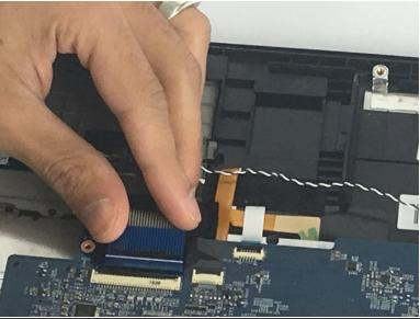
Gently lift the selected black tab that connects the cable onto the board and then slide out the cable.
