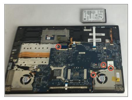
Remove the four 2.5 mm screws from the motherboard.
