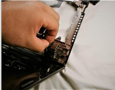
• lift up power jack and remove from holding tabs
