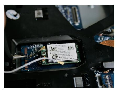
• Remove wifi wires by lifting up
