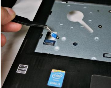
• lift clip to remove power button ribbon cable.
