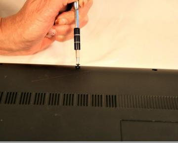
Remove the three screws securing the outer cover of the laptop using a Phillips #0 screwdriver.
