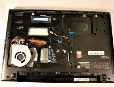
Slide the cover away from the hinges and lift the panel off.
