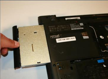
Remove the CD Drive fixing screw (#00x5.5mm) and slide the drive out from it's slot.
