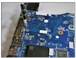
• Remove the three motherboard fixing screws (#00x5.5mm) and remove the motherboard.
