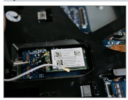
Use tweezers to carefully remove the white and black wires from the WiFi card. Thread the wires back out of it's channel and hold to the side.
