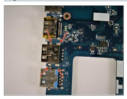
These joints will have to be soldered for removal
