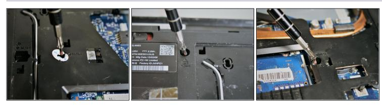
• Remove the three #00x5.5mm screws holding the keyboard.
