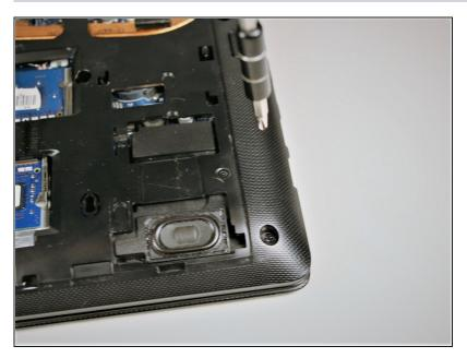
Remove the six perimeter #00x5.5mm screws holding the palm rest.
