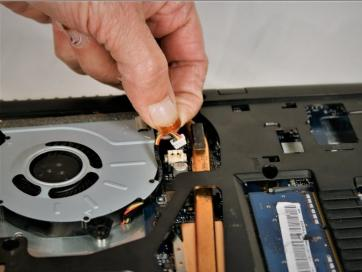
• Remove the three #00x5.5mm screws from the fan unit, unplug the fan wiring connector and then remove the fan unit.
