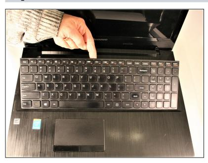
• Flip the laptop over, lift the screen and with a plastic spudger begin to remove the keyboard. Start at the top left corner and work from left to right lifting the keyboard. Once the top section is free, lift the keyboard up and away from yourself. Remove the ribbon cable connection and set the keyboard aside.
