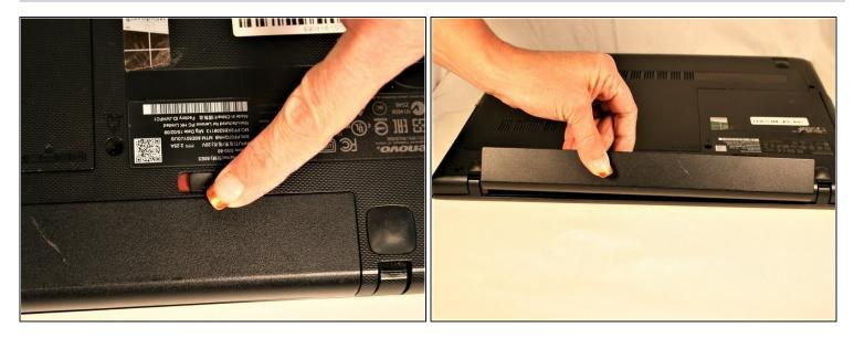
• From the underside of the laptop, press the two battery tabs inward to remove the battery. Lift the battery to remove.
