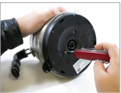
Reattach the base of the kettle to the steel body, while making sure the newly repaired wire does not come undone.
