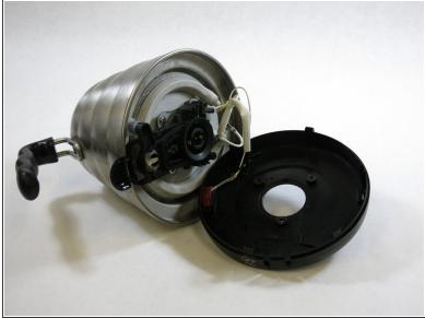
Detatch the base of the kettle from the steel body, exposing the internal wires.
