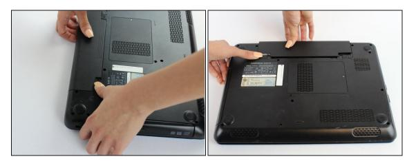
• While holding the left-hand switch to the left position, pull the battery away from the laptop.
