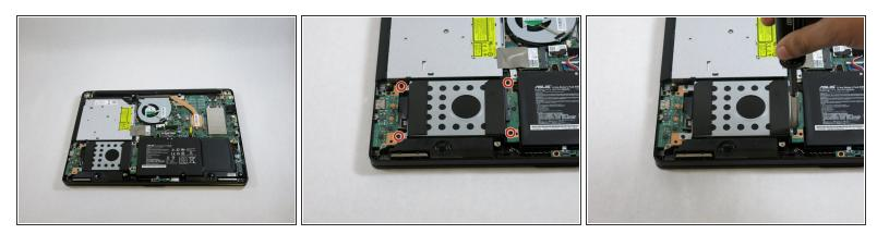
• Use a Phillips #1 screwdriver to remove the four 3.0 mm Phillips screws around the hard drive.
