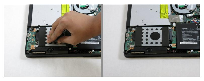
• Remove the hard drive from its port by sliding the hard drive left.
