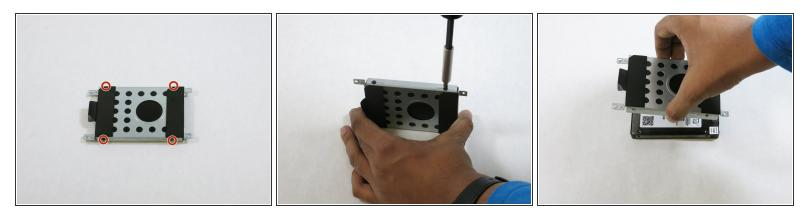
Use a Phillips #1 screwdriver to remove the four 2.0 mm Phillips screws that secure the hard drive to its casing.
