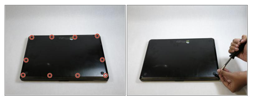
Use a T5 (Torx 5) screwdriver to remove the ten 3.0 mm Torx screws from the base plate of the laptop.
