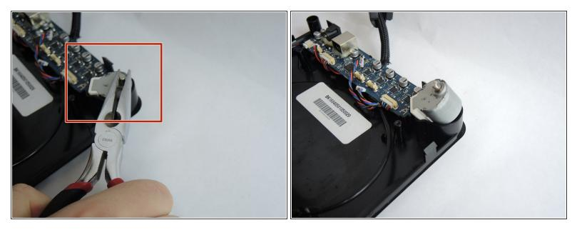
Once disconnected you will proceed to lift the motor using pliers.
