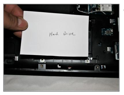
With the screws removed, slide the hard drive away from the center of the laptop and remove it.
