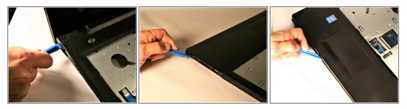
• Disconnect the two ribbon cables then using a plastic spudger, begin to separate the the palm rest from the chassis. Start along the front left edge and work left to right to separate each half. Separate the left and right sides in the same fashion.
