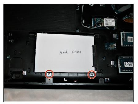
• Remove the two #00x4.5mm screws from the hard drive and then slide the drive to the side and remove the hard drive.
