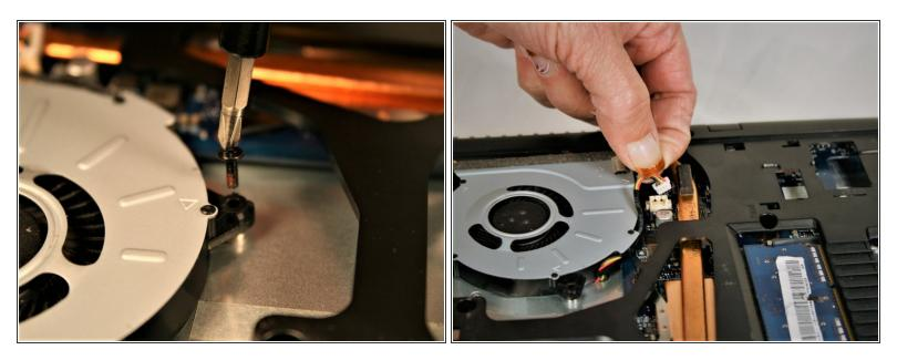
• Remove the three #00x5.5mm screws from the fan unit, unplug the fan wiring connector and then remove the fan unit.
