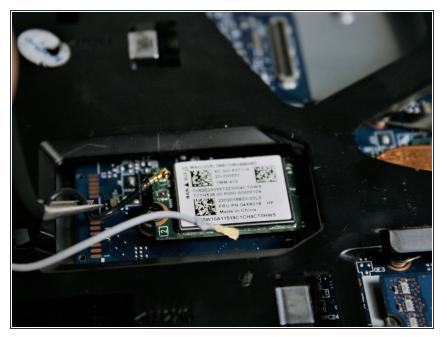
Use tweezers to carefully remove the white and black wires from the WiFi card. Thread the wires back out of it's channel and hold to the side.
