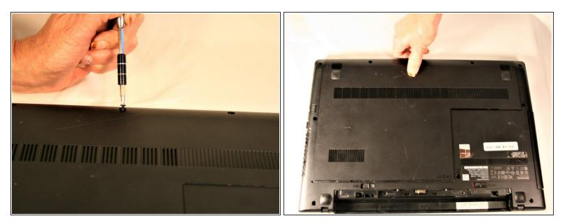
Remove the three #00x5.5mm screws from the bottom front under panel and then slide the main access panel forward and out.
