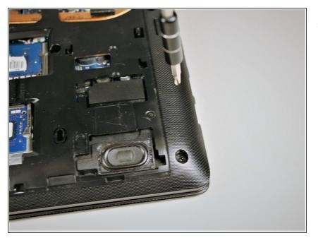
Remove the six perimeter #00x5.5mm screws holding the palm rest.
