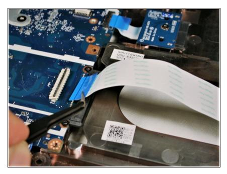
• Unplug the two ribbon cables from under the fan unit area.
