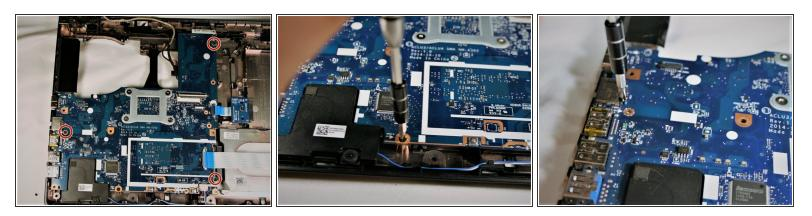
• Remove the three motherboard fixing screws (#00x5.5mm) and remove the motherboard.
