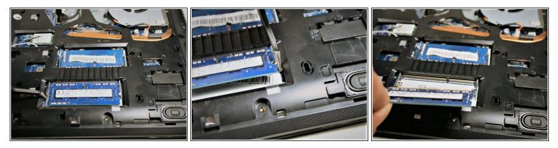
• Release the RAM fixing clip from both ends of each RAM chip. Once released, slide out each RAM chip.
