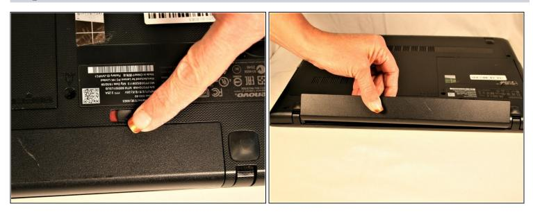
• From the underside of the laptop, press the two battery tabs inward to remove the battery. Lift the battery to remove.
