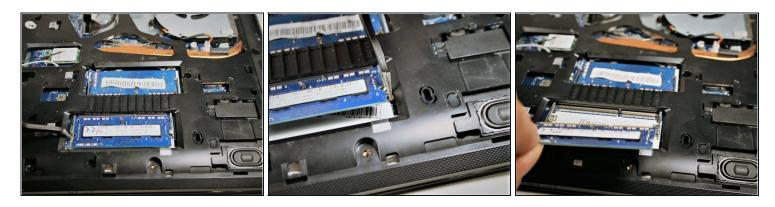
• Release the RAM fixing clip from both ends of each RAM chip. Once released, slide out each RAM chip.
