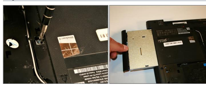
• Remove the CD Drive fixing screw (#00x5.5mm) and slide the drive out from it's slot.
