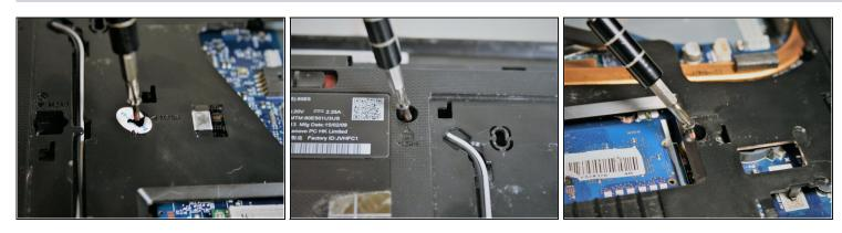
• Remove the three #00x5.5mm screws holding the keyboard.
