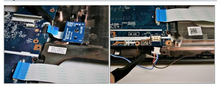
• Disconnect the CD Drive ribbon cable and the auxiliary board cable. Disconnect the speaker cable and then remove the CD Drive board fixing screw (#00x4.5mm). Remove the auxiliary board fixing screw and then remove the auxiliary board.
