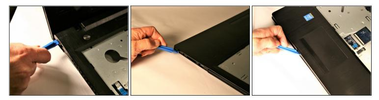
• Disconnect the two ribbon cables then using a plastic spudger, begin to separate the the palm rest from the chassis. Start along the front left edge and work left to right to separate each half. Separate the left and right sides in the same fashion.
