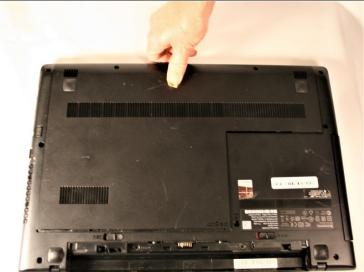
• Remove the three #00x5.5mm screws from the bottom front under panel and then slide the main access panel forward and out.
