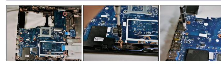
Remove the three motherboard fixing screws (#00x5.5mm) and remove the motherboard.
