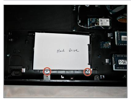
Remove the two #00x4.5mm screws from the hard drive and then slide the drive to the side and remove the hard drive.
