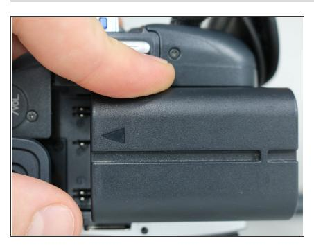
Pull the battery towards the bottom of the camcorder while lifting battery
