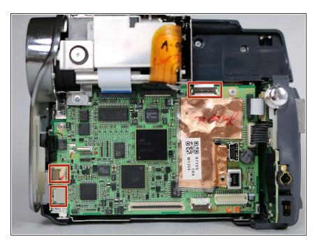
Unplug the three cables from the circuit board.
