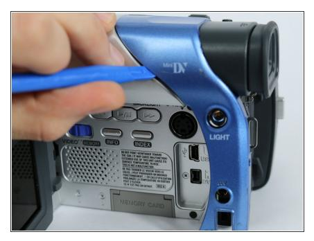
Use the small plastic opening tool to remove the blue side cover piece.
