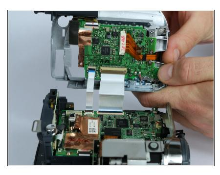
Gently pull apart both halves of the camera to reveal the inner components.
