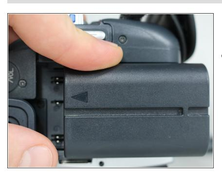
Pull the battery towards the bottom of the camcorder while lifting battery
