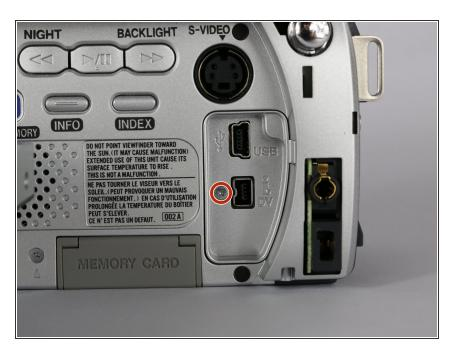
Remove the 3.1 mm screw next to the USB and DV inputs.
