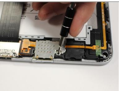
Remove the one 3mm Phillips #00 screw connected to the SD port.
