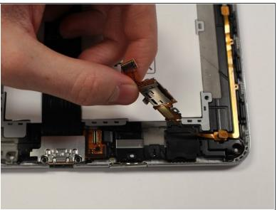
Using the orange tab, pull the SD port up and away from the device.
