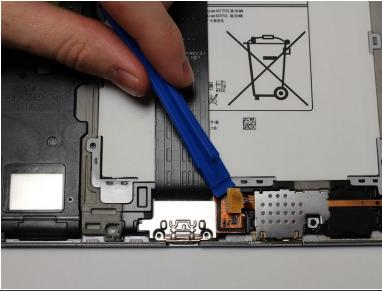
Pop up the orange tab connected to the SD port with the plastic opening tool.
