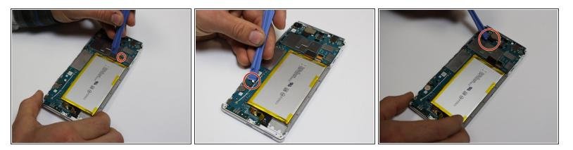
Disconnect all four of the shown electrical connectors by gently prying up with the plastic opening tool.
