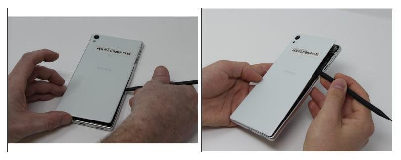
• Carefully remove the back panel of the phone with a plastic spudger, or other flat and thin wedge tool. Work your way around the perimeter of the case, loosening and prying gently, until there is sufficient distance between the panel and phone.
