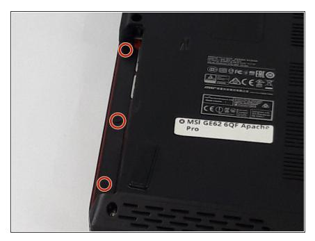
Use a Phillips screwdriver to remove the three screws along the edge of the optical drive bay.
