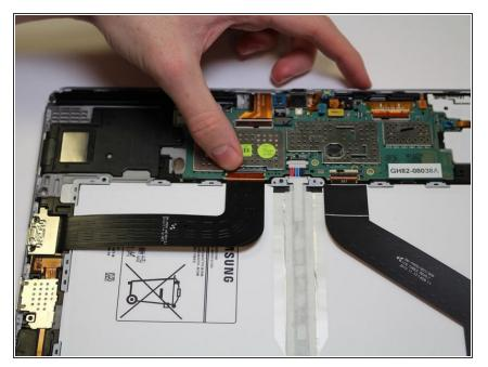
• Using your finger, push up on the clip to disconnect from the device.
