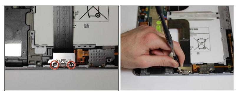
Remove the two 3mm screws from the silver cover using the Phillips #00 screwdriver.
