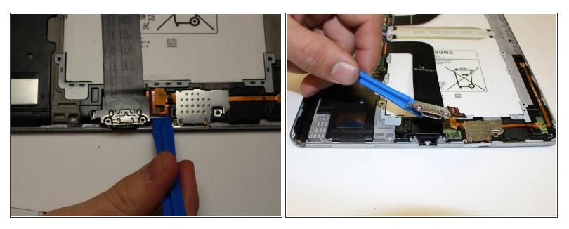
• Using the plastic opening tool, carefully lift away the orange piece connected to the USB port.
