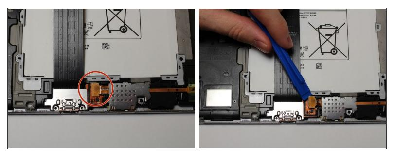
Pop open the orange tab that is connected to the SD port using the plastic opening tool.
