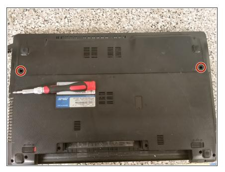
Remove the two Philips screws securing the RAM cover.
