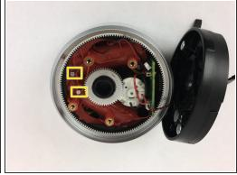
Grab the gears and lift them up to remove from the device
