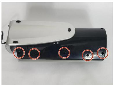
Start off by using a Philips #2 screwdriver to remove all eight 10mm exterior screws on the rear of the device.
