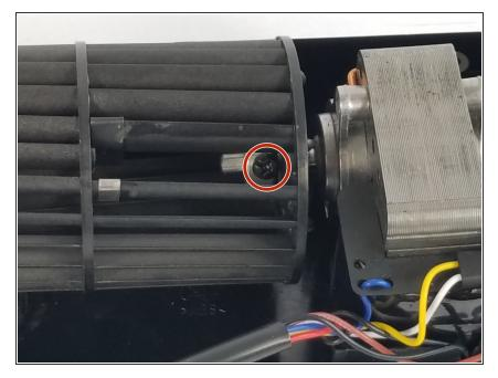
Loosen 5mm #2 screw at bottom of fan blade.
