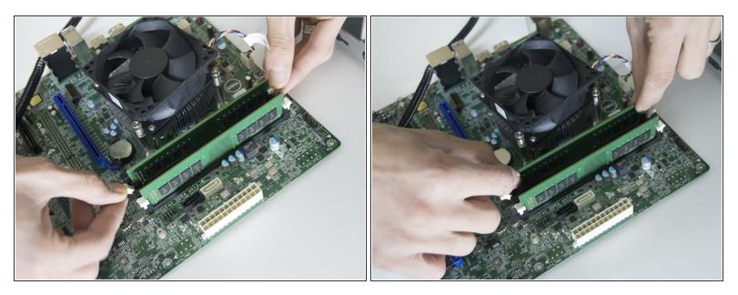
• Now, carefully remove each RAM from its slot by pushing down the tabs as shown.
