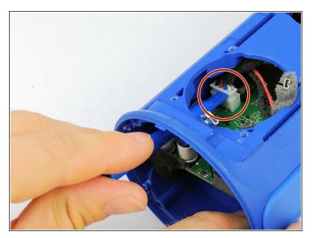
Remove the speaker wires from the control panel by prying off with a plastic opening tool.
