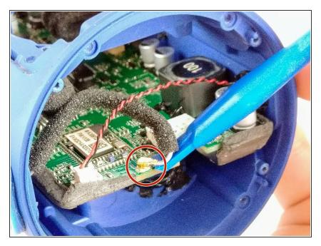
• Use a spudger to disconnect the gold antenna connector from the main circuit board.
