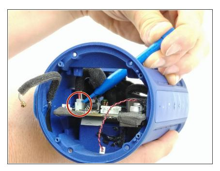
Disconnect micro-b connector with a plastic opening tool.
