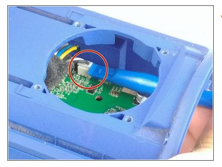
Use a plastic opening tool to disconnect the 3.5 mm headphone connector.
