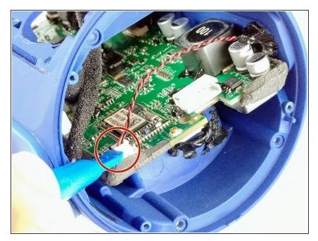
Disconnect the microphone connector using the plastic opening tool.
