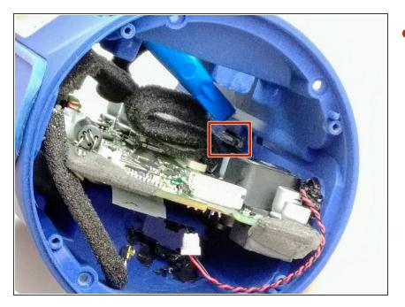
Next, disconnect the control-panel ribbon by prying out the grey plastic tab using a plastic opening tool. The ribbon should freely come out afterwards.
