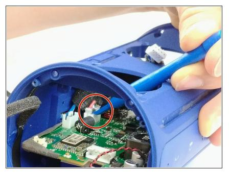
Remove the connector to the USB connector using a plastic opening tool.
