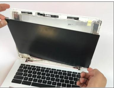
Using the JIS J000 Screwdriver, unscrew and remove the (4) four 3mm screws from the display.
