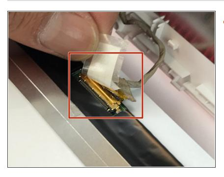
Gently peel back the tape to remove the display.
