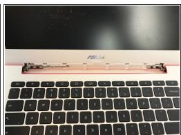
Flip open the Chromebook as shown. Using the plastic opening tool, gently pry open the hinge cover of the display. Once it snaps off, remove the hinge cover.
