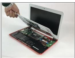
Gently wedge the spudger in between the bottom of the device and the keyboard, and carefully pry
