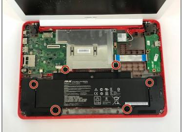
• Using the JIS-J0 Screwdriver, remove the (6) six 6 mm screws from the battery.
