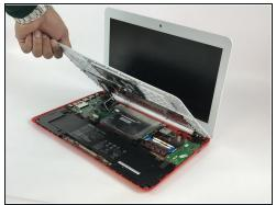
• Gently wedge the spudger in between the bottom of the device and the keyboard, and carefully pry the cover open. Then, carefully lift up on keyboard.
