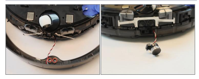
• Flip the Roomba back over and unscrew the 2 screws that connect the sensor to the bumper.
