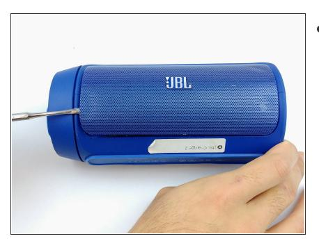
Remove the opposite screen cover using a metal spudger
