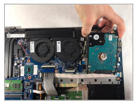
Lift the hard drive up to remove from the device
