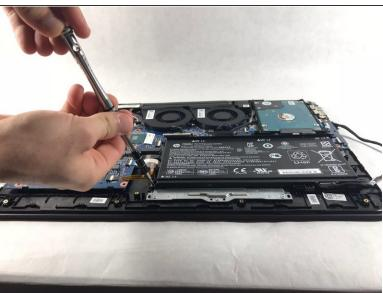
Remove the four 1.2 mm Phillips #00 screws around the battery.
