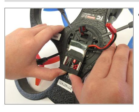
Push the battery upward with your thumbs to loosen it from the tight slot until your thumbs can not reach the bottom of the battery anymore.
