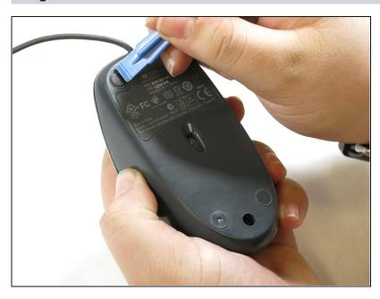
After re-assembling the mouse, don't forget to reattach the mouse feet onto their correct locations on the bottom of the mouse.
