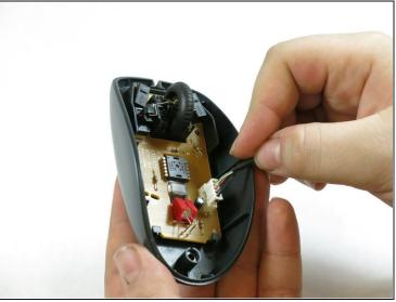
• Take the replacement USB cable and connect it to the mainboard.
