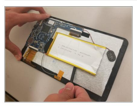
Insert plastic spudger underneath the edges of the battery to pry it up and detach the adhesive.
