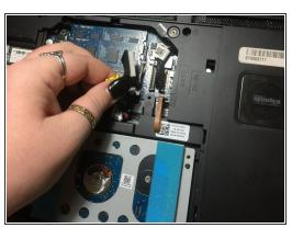
Carefully unplug the black cord with the yellow tag to disconnect the battery.
