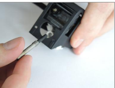
To remove the nozzle, use a 5 mm nut driver to unscrew it.
