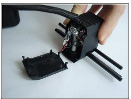
Slide the tracks off the second slider and remove the printer head and x-tracks from the center of the printer. To remove the front cover of the print head, firmly grip the cover and gently pull it off.
