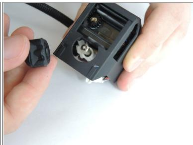
• To remove the nozzle insulation, grip the insulation and pull it up off of the nozzle.
