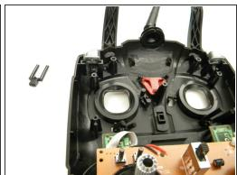
Remove the trim rocker switch from the controller.
