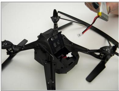
Disconnect white connectors between the battery pack and drone.
