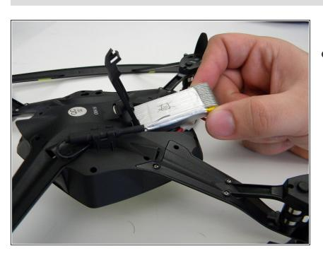
Remove battery pack from body of drone.
