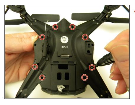
Remove the eight (8) 5mm Philips screws attaching the motor arms to the body using a Philips J00 screwdriver.
